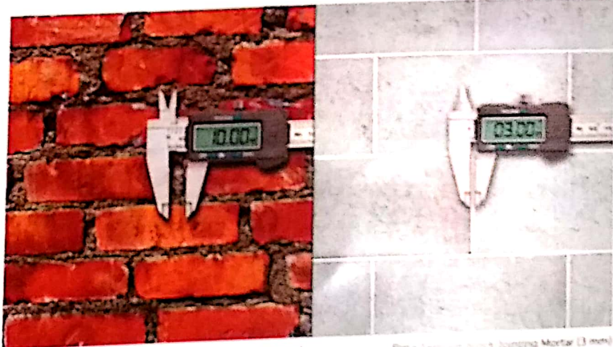
Traditional mortar joints (10 mm)
